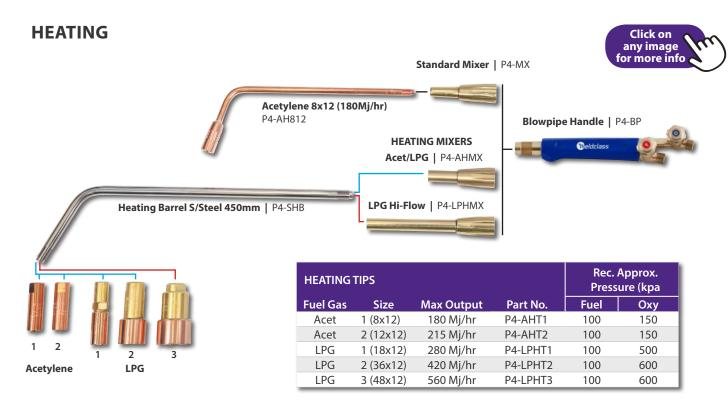
**Handy Tip:** Heating with Oxy/Acetylene become unsafe when drawing large flows from the acetylene cylinder (eg: during heavy & very heavy heating). For this reason, Oxy/Acetylene heating tips are not available in large / very large sizes, as indicated above. Oxy/LPG does not have the same restriction & Oxy/LPG heating tips are available in larger sizes for heavy heating applications. Overall, Oxy/LPG is safer and less costly than Oxy/Acetylene.
