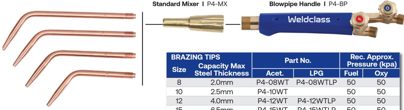
**Handy Tip:** Oxy brazing can be done with both Oxy/Acetylene and Oxy/LPG. Oxy welding (eg welding steel together using steel filler wire), is only possible with Oxy/Acetylene.
