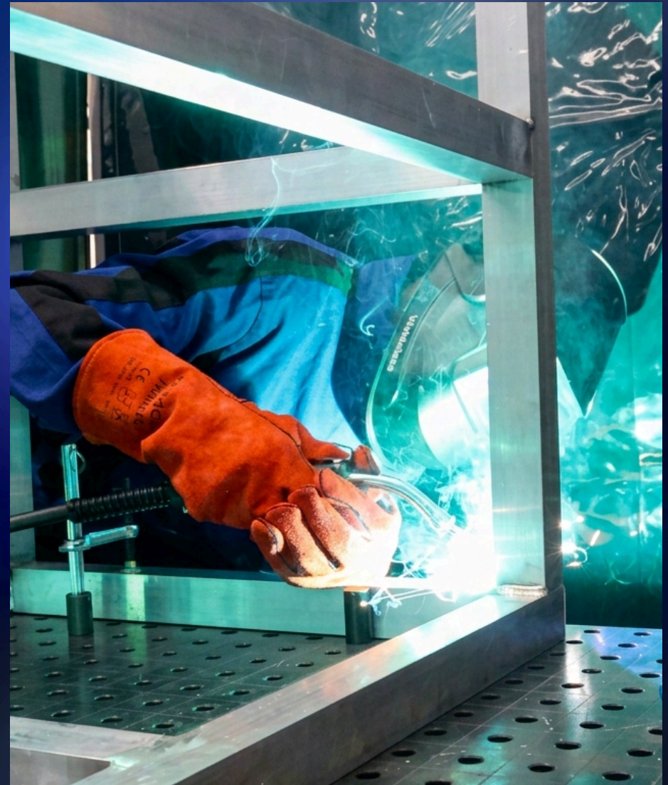
3mm Aluminium Sheet welded with FURY 185 MPST using 1.0mm AL5356 Wire and Pure Argon Shielding Gas at 145-Amps
