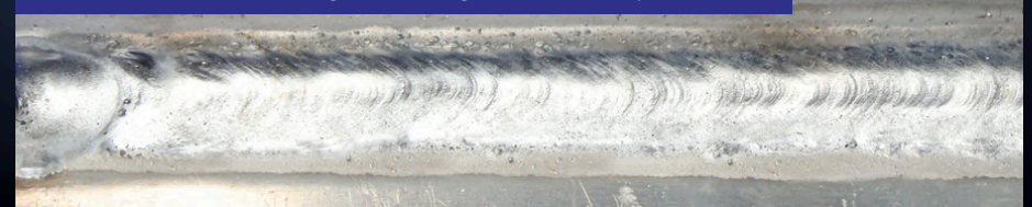
3mm Aluminium Sheet welded with FURY 185 MPST using 1.0mm AL5356 Wire and Pure Argon Shielding Gas at 145-Amps
